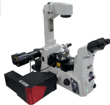
K1-Fluo with commercial microscope
